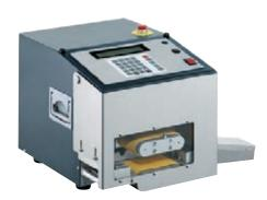
The CCM microprocessor-controlled automatic cutter cuts to length ribbon cables, round cables, insulating conduits and tubes. Its high repeat accuracy is achieved using a precision AC servodrive. The dimensional accuracy can, for particular requirements, be optimised by means of length correction.
