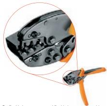
For flat-blade connectors and flat-blade receptacles with pre-rolled crimp claw
