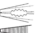
Telegraph pliers (combination pliers) acc. to DIN 5746
